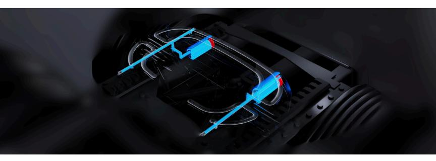
• Grease fills the grooves on the top plate of the fifth wheel.
